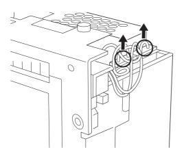
5) Disconnect the backlight's two (2) power connectors.
