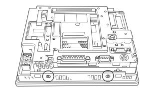
3) Remove the unit's four (4) top and bottom face attachment screws (Figure shows bottom face screw locations - top face locations are the same).
